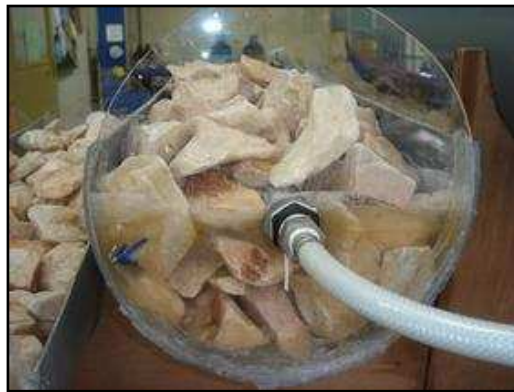
Fig. 3. Armouring due to iron precipitation in open limestone channel
